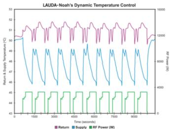
The 300mm chamber temperature profile comparison above illustrates the performance of LAUDA-Noah's dynamic POU system vs. a static unit on an etch process. Perhaps the most compelling aspects of this data set are the temperature uniformity and rapid response times accomplished under these extremely high RF power conditions.
