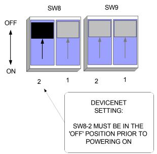
Figure 3-2. DeviceNet Switch Setting Diagram
