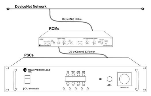
Figure 3-4. DeviceNet™ Connection Block Diagram
