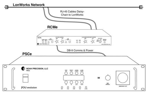
Figure 3-3. LonWorks™ Connection Block Diagram
