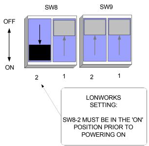
Figure 3-1. LonWorks Switch Setting Diagram
