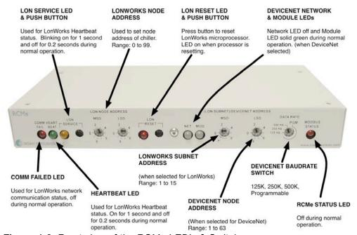
Figure 1-2. Front view of the RCMe LED's & Switches
